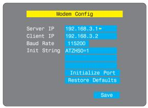
The default items here are perfectly adequate for the majority of modem and ISDN terminal adapter installations.
